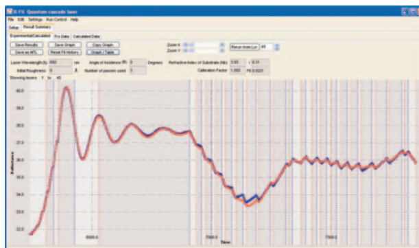
With R-Fit ® v4, you can fit layers of only a few Angstroms thickness.
